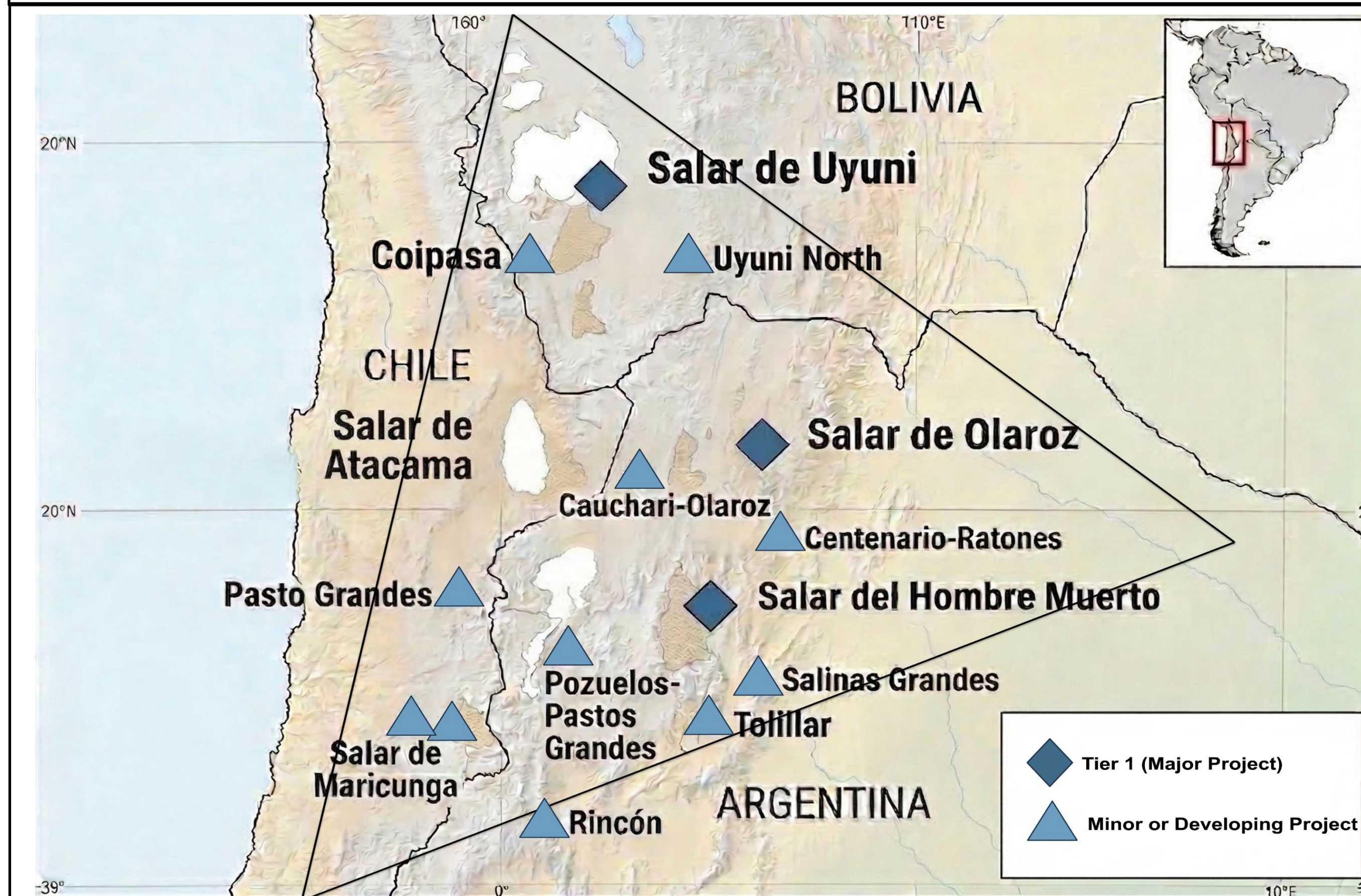
Figure 3: The Lithium Triangle with major and minor lithium mining projects. Tier 1 mining projects generate over $300 million USD annually, have lithium reserves to sustain 20+ years of operations, and sit in the bottom quartile of the global mining cost curve (Schodde 2013).
